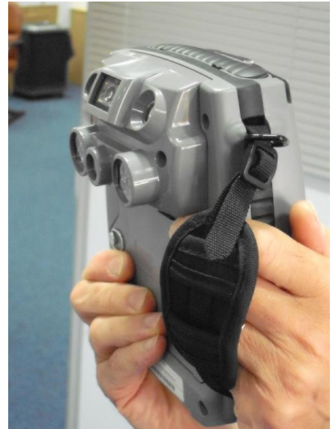
Example: Datastrip's DSV3 Multi-modal mobile reader incorporates MIRLIN Iris Recognition Engine with TRIAD application software
